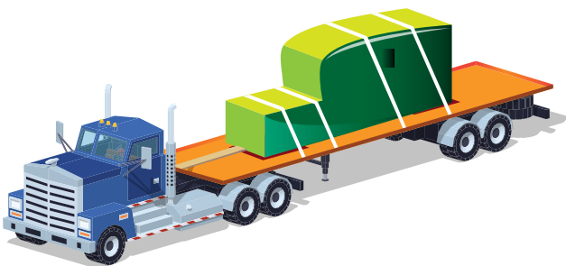
Simple top over lashing
