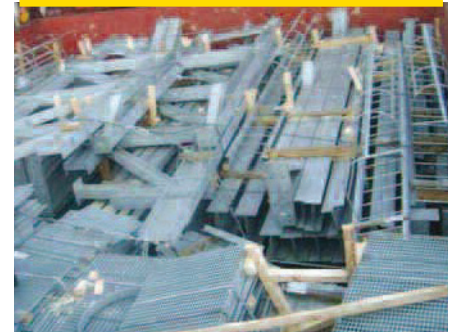
Full cargo hold with inadequate dunnage, showing little regard to the weight imposed on the lower tiers
