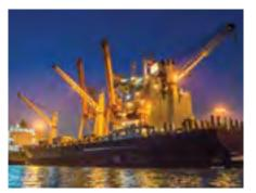
A heavy-lift vessel specifically designed for the carriage of heavy project cargo. Two cranes allow for tandem lifts.
