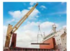
A single, heavy-lift derrick on a cargo vessel poses limitations on the lifting of long columns.
